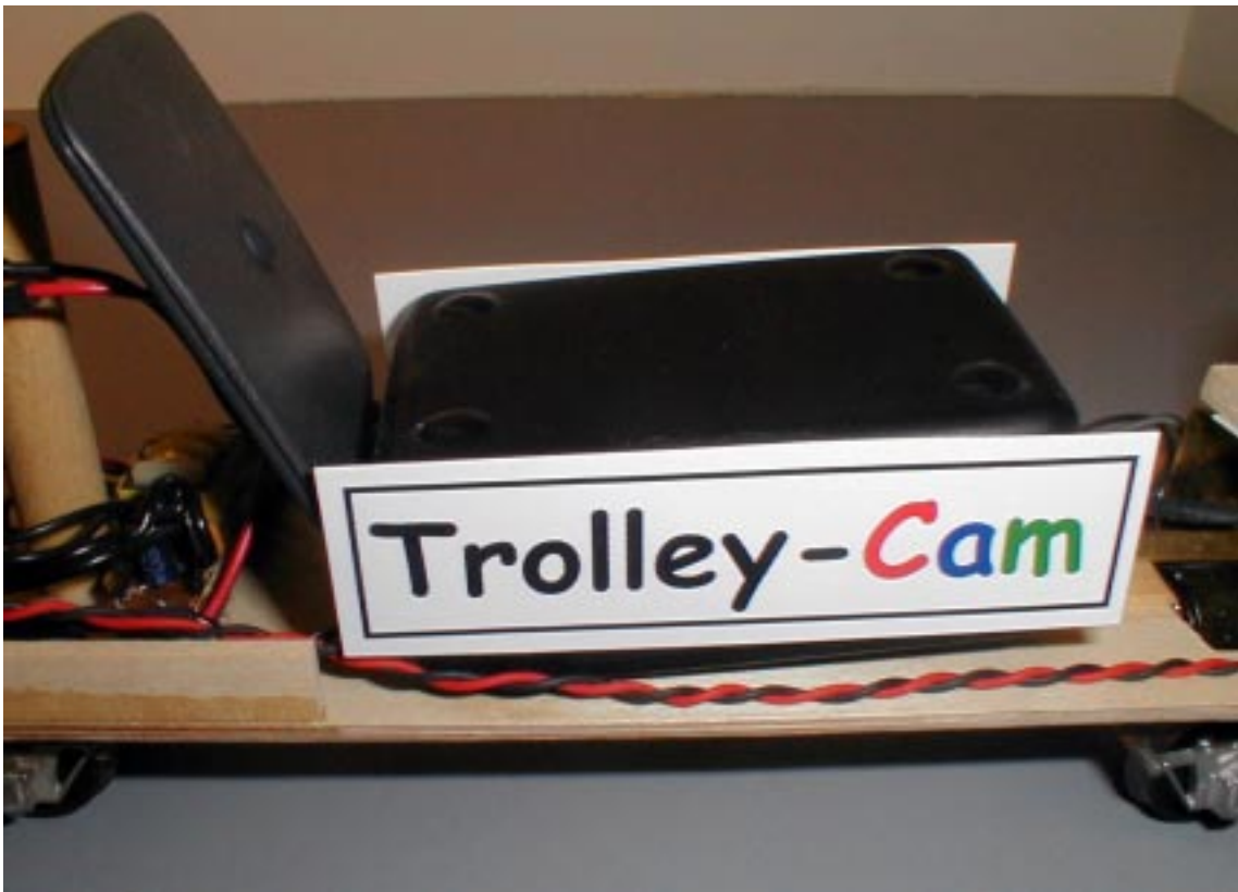
Photo 5 – This view shows the camera circuit board mounted in its new, smaller box. The flat panel sticking up behind the box is the antenna.
